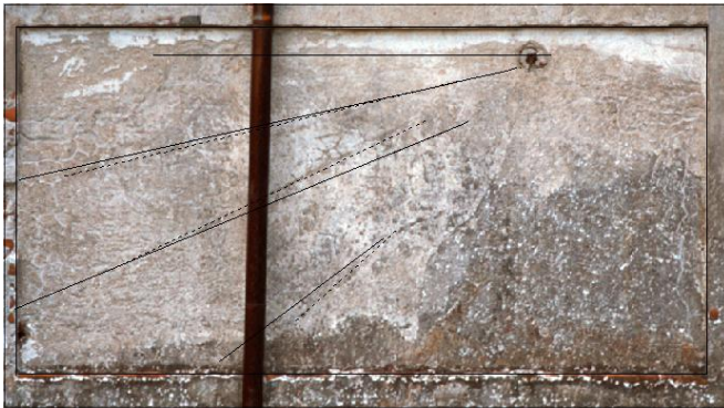
Fig. 11. Dial no. 6; lines still visible (dotted line) and computer reconstruction (full line) are marked.
